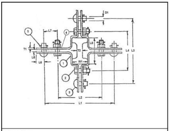
DIMENSIONS IN MM : POLE MOUNTED STAY CLAMP (RAIL)
